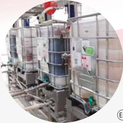
**(EN)** A single unit for the preparation of finished syrup or drink, by in-line and continuous dosing and mixing of 2 to 6 ingredients. Automatic recipe management and automatic control of all working parameters. Outlet °Bx variation (steady production)  $\sigma = 0.02^\circ\text{Brix}$ . Total recovery of concentrates and final product.
