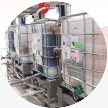
**(EN)** A single unit for the preparation of finished syrup or drink, by in-line and continuous dosing and mixing of 2 to 6 ingredients. Automatic recipe management and automatic control of all working parameters. Outlet °Bx variation (steady production)  $\sigma=0.02^{\circ}\text{Bx}$ . Total recovery of concentrates and final product.
